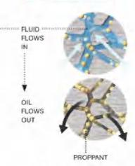
Fracking fluid expands cracks in the rock, releasing oil, which flows back up the well.
